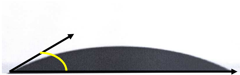
Untreated ceramic tile Contact angle: 38°
