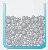
With their low surface area to volume ratio, 3M ceramic microspheres can help reduce resin demand and increase volume loading capacity. Smaller particles help fill voids between larger ones for high packing density.
