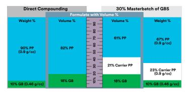
Figure 2. Directly Compounded 10% 3M<sup>™</sup> Glass Bubbles vs. Masterbatch Addition of 3M<sup>™</sup> Glass Bubbles – Carrier Resin wt. and Vol. % Implications.
