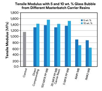
Figure 5. Tensile Modulus Changes with Different Masterbatch Carrier Resins
