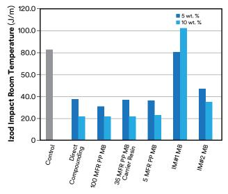
Figure 7. Room Temperature Izod Impact Changes with Different Masterbatch Carrier Resins
