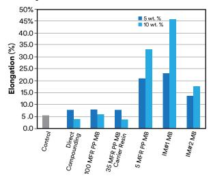
**Elongation with Different Masterbatch Carrier Resins**
