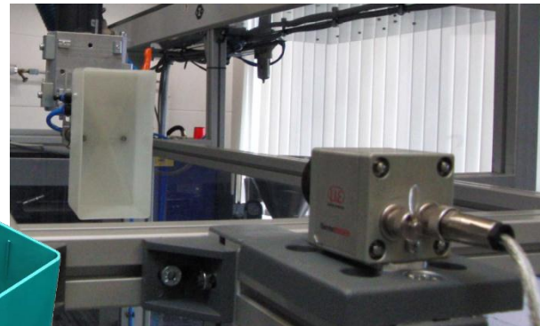
Experimental Setup: Ejection Temp measured by IR
